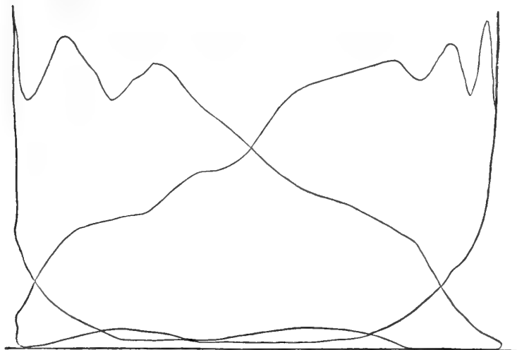
Fig. 13.—Indicator Diagram of the after cylinder of Messrs. Ransomes, Sims, and Head's 8-Horse-power Farm Steamer, No. 2149.
