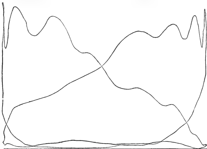
Fig. 13.—Indicator Diagram of the after cylinder of Messrs. Ransomes, Sims, and Head's 8-Horse-power Farm Steamer, No. 2149.
