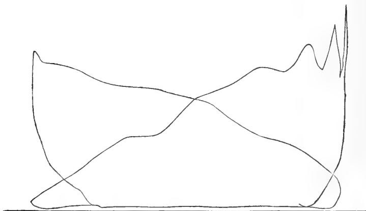
Fig. 7.—Indicator Diagram of Messrs. Aveling and Porter's 6-Horse-power Locomotive, No. 7002.
