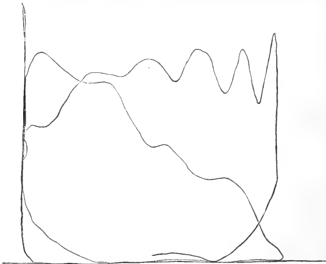
Fig. 14.—Indicator Diagram of the right-hand cylinder of Burrell's 8-Horse-power Thomson's Patent Locomotive, No. 3661.
