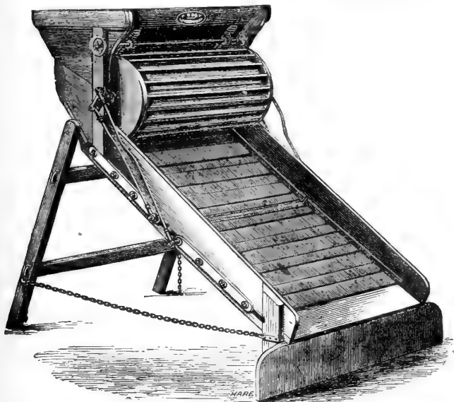
Fig. 32.— Boby's New Patent Self-acting Corn Screen.
