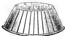
A single disc, as used in the "Alpha" machines and in the "Leviathan."
