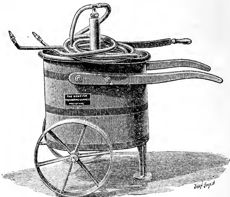
FIG. 8.—A Hand Hop-washing Machine.
