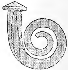
FIG. 6.—Bent Steel Nail.
