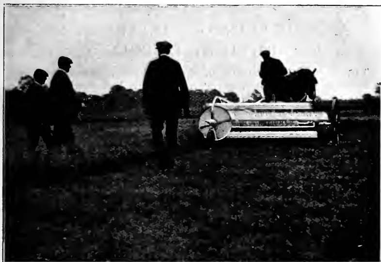
FIG. 5.—Martin's Side Delivery Rake making a Wagon-row.
