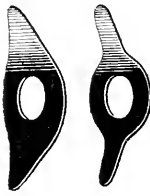
FIG. 4.—Two curved, perforated, steel springs made from thin, safety-razor blades, as described in the text. These two forms, while of the same length, nearly 1 in., are of different degrees of springiness; that at the left being the weaker.
