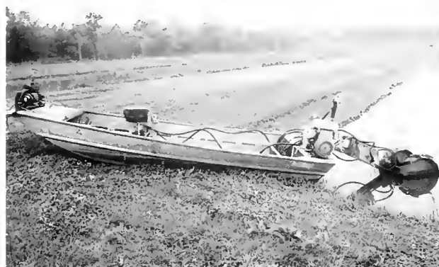
Figure 4. Crawfish harvest boat, "crawfish combine" design.
