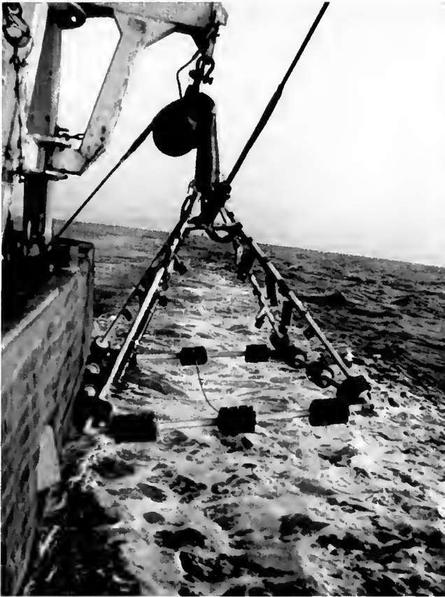
Figure 1. The SMAST video sampling pyramid aboard the F/V Huntress . The pyramid has a square base 2.2 m per side of 6 cm round iron, arms 2.5 m \times 4.5 cm round iron and weighs approximately 450 kg. It is deployed with the large hydraulic winch used in the scallop fishing industry while a second tension sensitive hydraulic winch controls the electronic cable. Rubber rings (three sets of eight rings, each 20 cm diameter, 5 cm thickness, per side) were placed on the base of this pyramid to prevent damage during deployment and provide gentle landings on the sea floor. Three underwater cameras (Deepsea Power & Light® multi-Seacam) and nine 100-w lights (Deepsea Power & Light® multi-Sealite) were attached to the pyramid.
