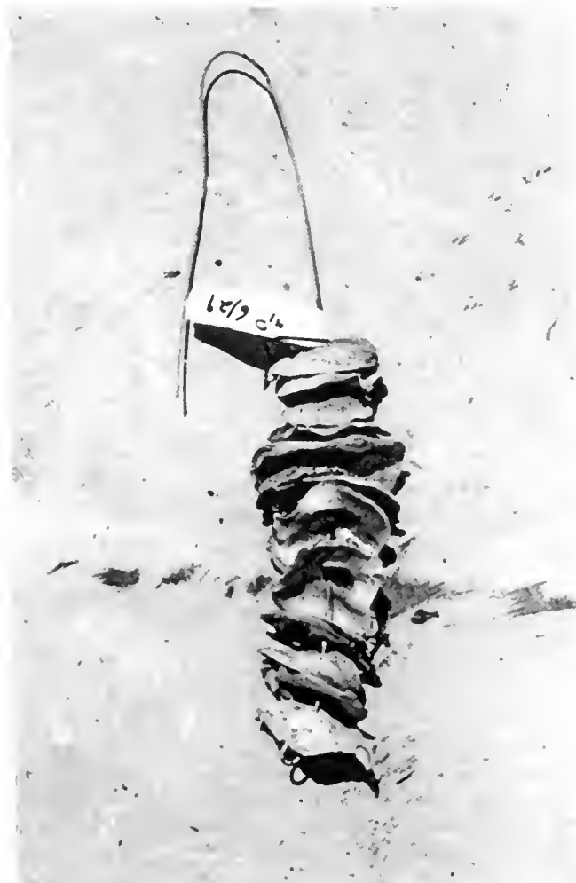
Figure 2. Picture of a typical shellstring used by the Virginia Institute of Marine Science Molluscan Ecology Program to monitor oyster spat settlement in Virginia estuaries, 1946 to present.
