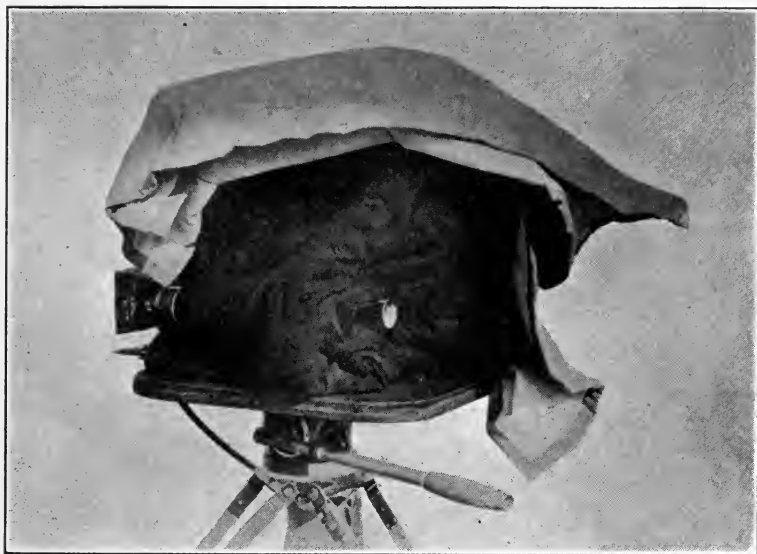
FIG. 4. A silencing camera cover.
