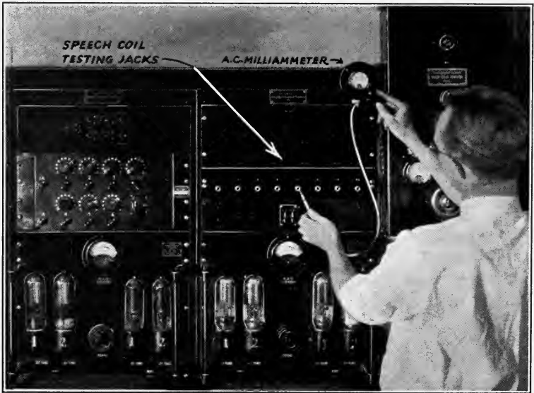
FIG. 3. Testing panel for detecting inoperative speech coil circuits in theater reproducing systems.
