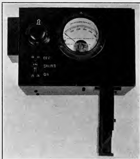
FIG. 5. Split beam light valve comparator device.
