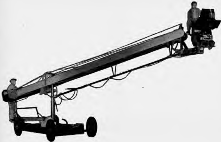
FIG. 1. The traveling camera boom.
