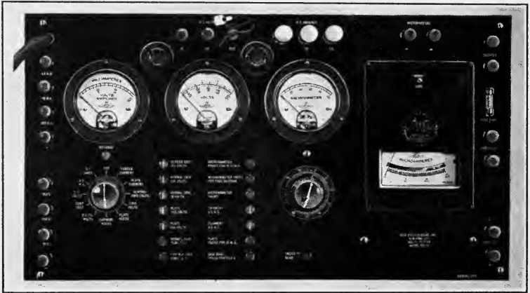
FIG. 3. Service engineer's multitester.
