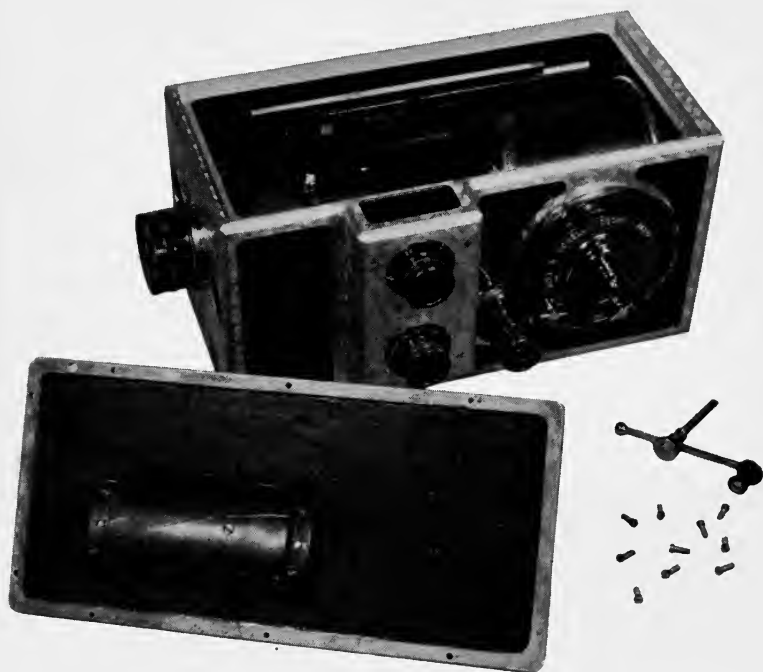
FIG. 4. Close-up showing interior of Varo lens. Note the four cams set in the cover, which operate the iris lever. These cams, from top to bottom, are for the settings of f /3.5, 4.5, 5.6, and 8, respectively.
