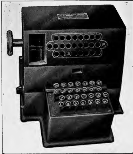
FIG. 1. Front view of the keyboard automatic light control, showing the keyboard, the scene numbering drum, and the recording indicator.
