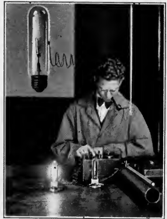
FIG. 9. Equipment for measuring bulb glass temperature.
