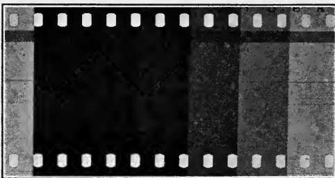
FIG. 2. Gammameter test strip with sound track.
