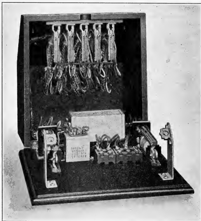
FIG. 6. Arrangement of apparatus in the five-unit control cabinet.
