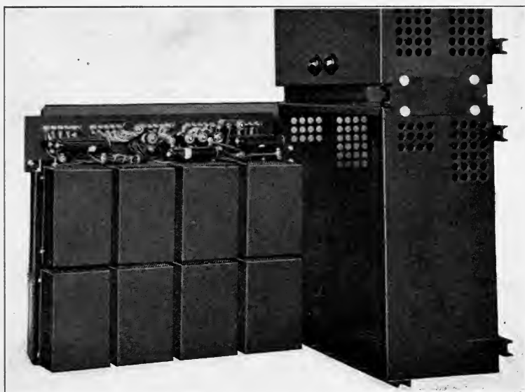
FIG. 7. View of lower section showing shielding.
