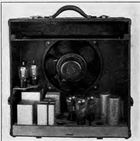
FIG. 6. Interior view of amplifier-loud speaker unit.
