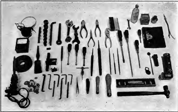
FIG. 2. Service engineer's kit of tools.
