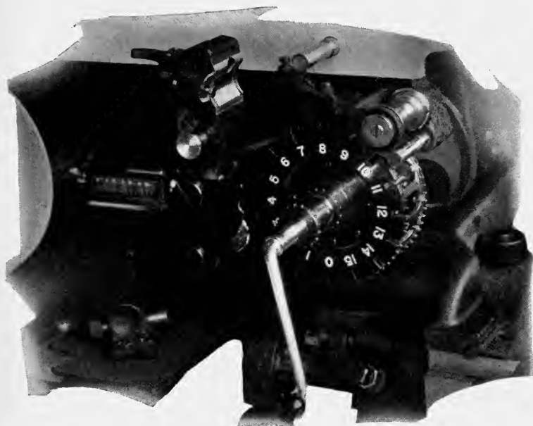
FIG. 10. B & H standard splicing machine with attachment to facilitate splicing matte films in exact synchronism with negatives.
