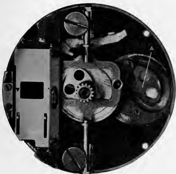
FIG. 4. Camera head mechanism; A , the cam that actuates the filter carrier.
