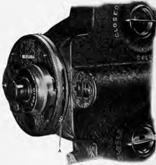
FIG. 3. Camera head showing slot through which color filters are inserted.
