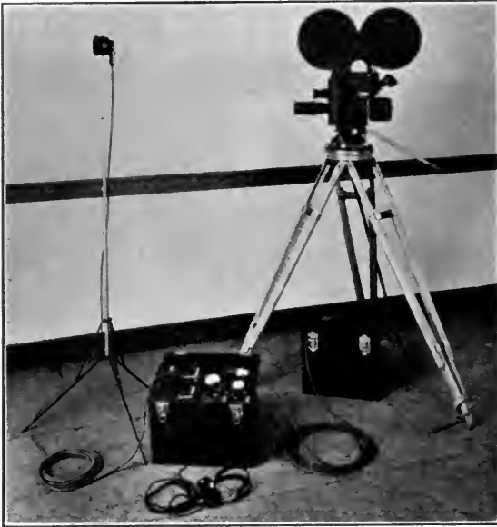
FIG. 4. Light-weight single-film recording system, complete with sound camera.
