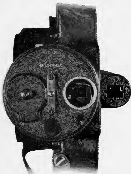
FIG. 2. Front view; lens removed showing oscillating filter.
