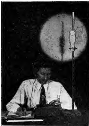
FIG. 8. A projector drum containing parabolic reflector, shown on test trunnion, which provides angular adjustment in vertical and horizontal planes.
