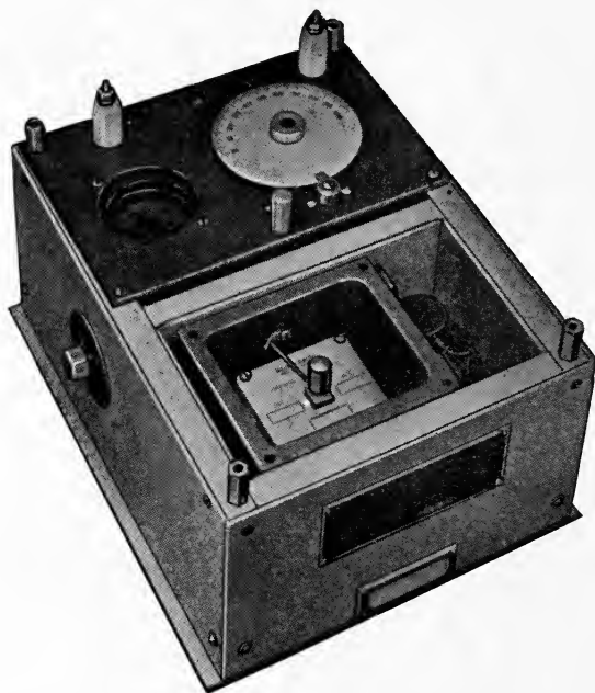
FIG. 8. Crystal frequency generator with cover removed, showing crystal holder and oven for controlling temperature.
