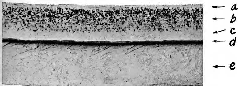
FIG. 1. Magnified cross-section of Superpan: (a) anti-abrasion coating; (b) first emulsion coating; (c) second emulsion coating; (d) gray-back coating; (e) base.
