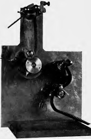
FIG. 5. A device for measuring film elastance.
