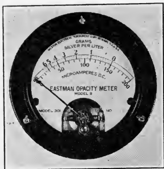
FIG. 3. The microammeter is calibrated directly in grams of silver per liter.
