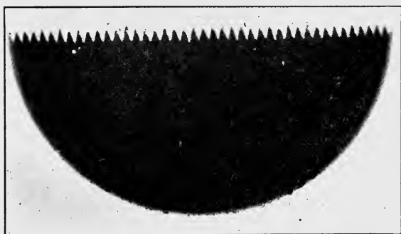
FIG. 9. Mechanographic sound-track showing resolution at 50,000 cps., at a recording level 55 db. below maximum.
