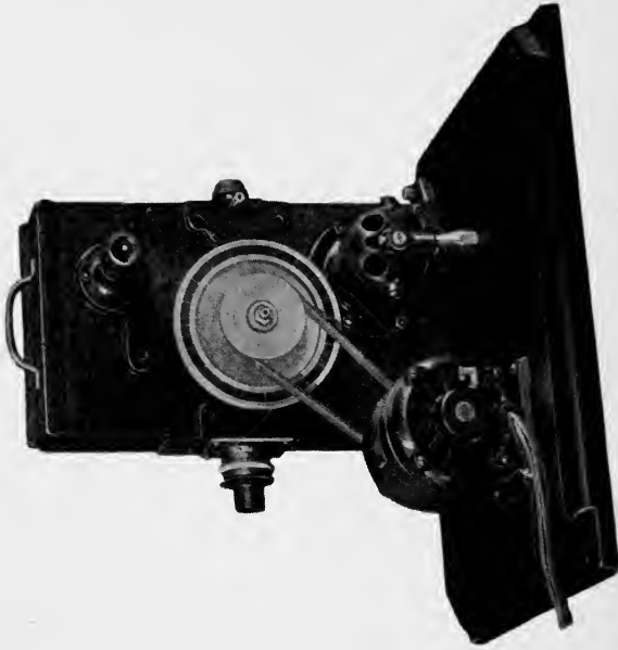
FIG. 4. Complete assembly of high-speed camera, showing driving motors and commutator.
