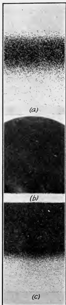
FIG. 5. Comparison of lines of demarcation between opaque and transparent sections of record; (a) photographic negative; noise reduction, zero modulation, variable-width; (b) mechanographic; zero modulation; (c) photographic positive; low modulation. 300x.
