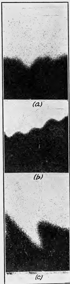
FIG. 8. Photographic copies, or prints, (a) from photographic sound-track; (b) from mechanographic sound-track; (c) from photographic sound-track. 300x.
