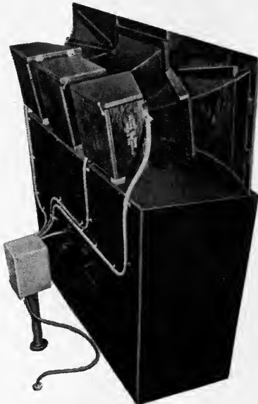
FIG. 3. Triplet and low-frequency loud speaker combination.
