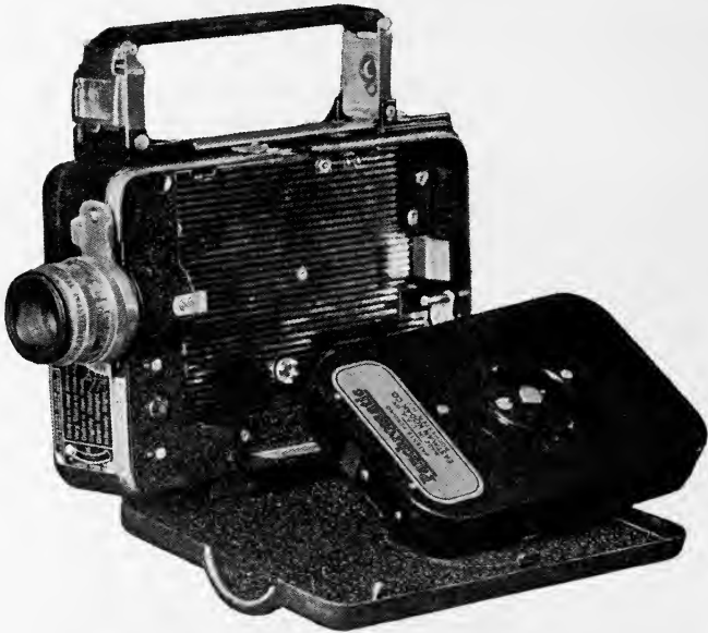
FIG. 3. Camera and magazine. (Note film indicator on magazine.)
