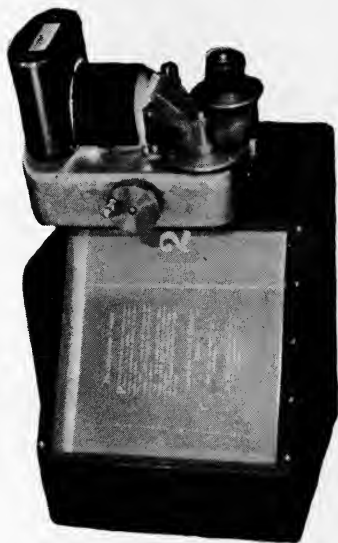
FIG. 4. Reading machine, showing 90-degree rotation of the head.
