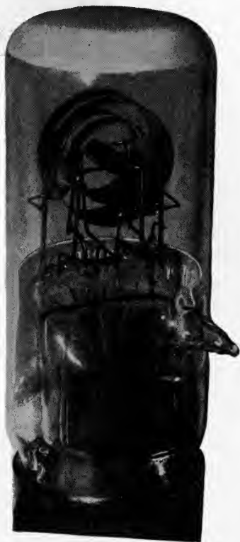
FIG. 3. Line-sound-film tube (normal product) with two cylindrical lenses in the electrooptical system.
