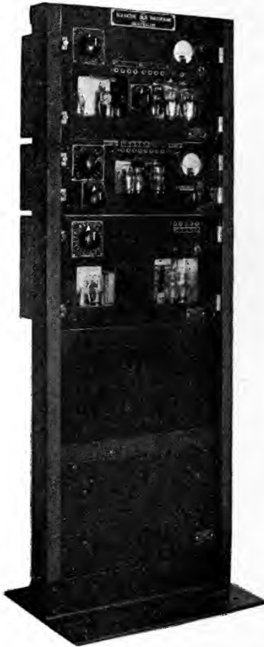
FIG. 5. Amplifier rack (tube covers removed).
