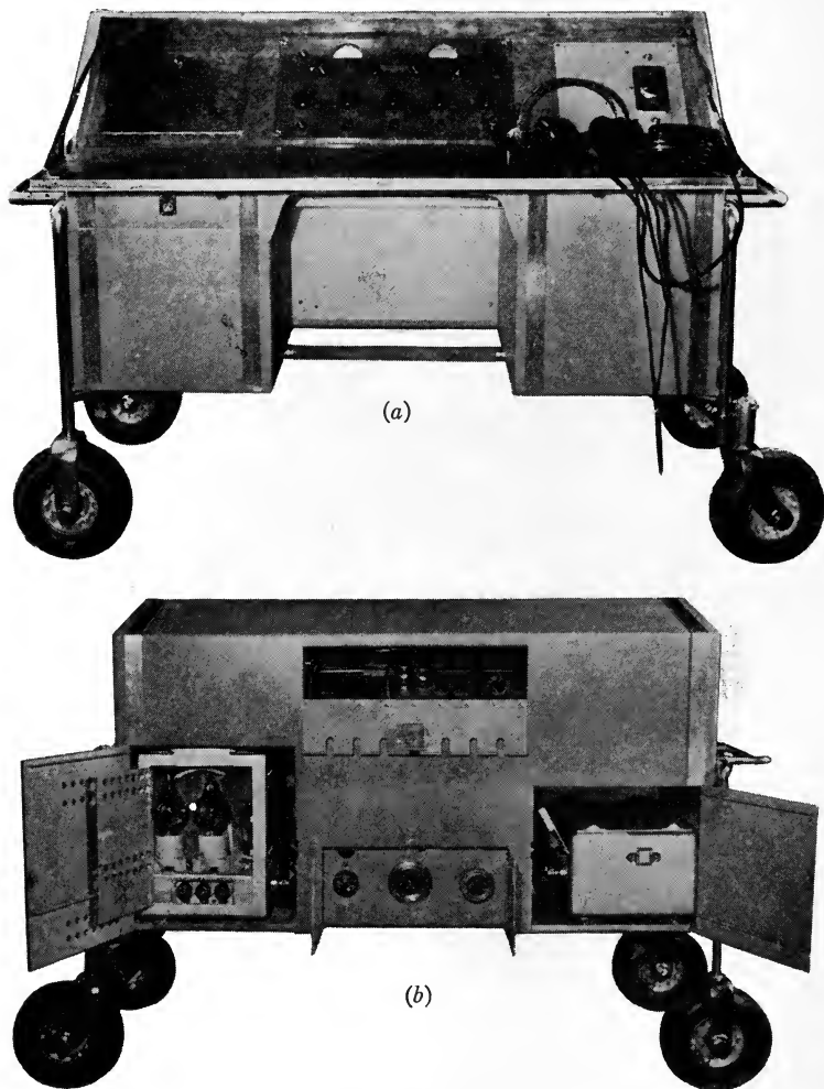
FIG. 12. Dolly-mounted portable ERPI recording system: (a) front view; (b) rear view ( Paramount Productions, Inc. ).
