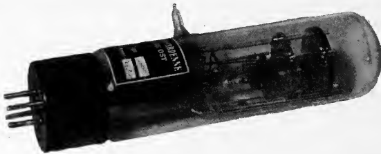
FIG. 2. Line-sound-film tube with combined variable-intensity and variable-amplitude characteristic.
