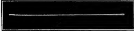
FIG. 4. Unretouched photograph of the fluorescent screen, showing the sharpness of the line and uniform intensity of illumination of the tube of Fig. 3.
