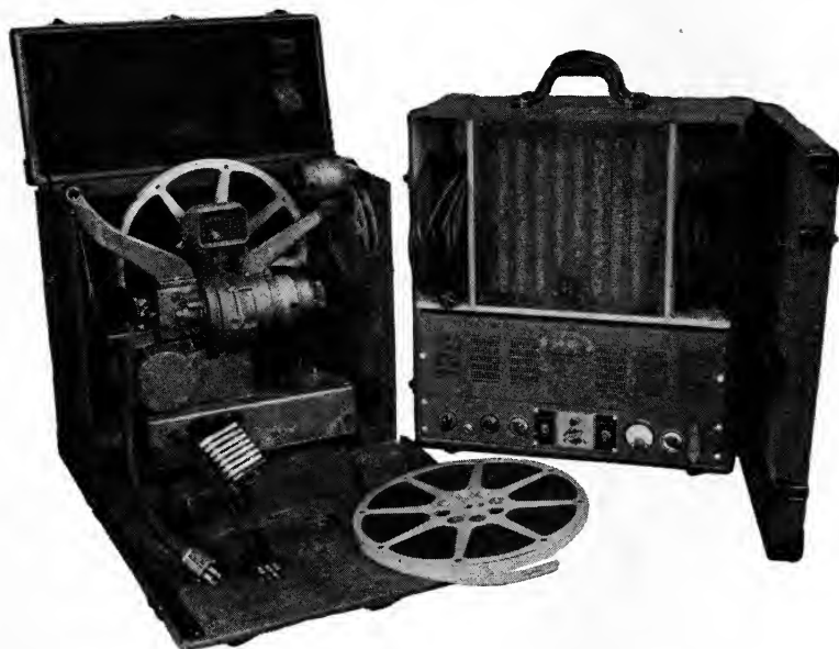
FIG. 1. 1000-watt 16-mm. Filmosound projector, with humidor unit removed to show arrangement.
