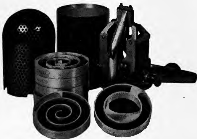
FIG. 14. Unassembled view of unidirectional microphone, showing pressure and velocity portions of the ribbon, magnetic structure, labyrinth, and pipe connecting pressure part of ribbon to labyrinth.
