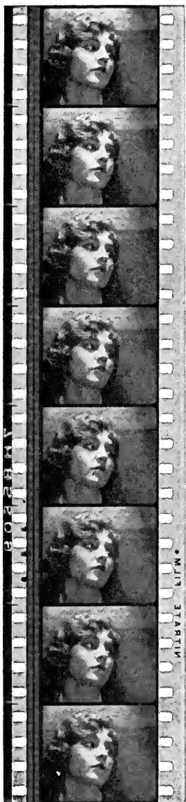
FIG. 3. Single variable-density double squeeze, showing transition from full-width track to double squeeze-track.
