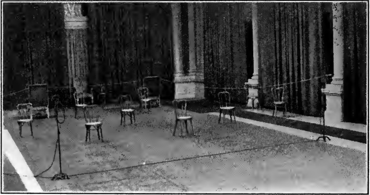
FIG. 6. Dummy stage used for testing accuracy of sound location.
