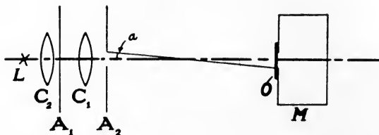
FIG. 2. Diagram of apparatus used for determining the Callier quotient.
