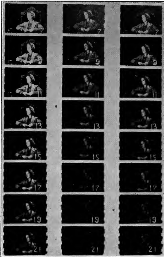
FIG. 10. Parts of three negative test-strips printed on positive film stock from (left) Ultra-Speed Panchromatic film exposed at stop f/4.5 ; (center) Superpan Negative film exposed at stop f/4.5 ; (right) Ultra-Speed Panchromatic film exposed at f/9 using a Fried light-tester.
