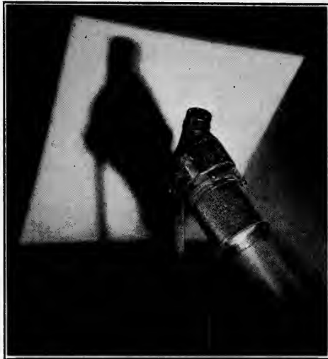
FIG. 15. Aperture spotlight lighted by means of a similar unit. Note the definite outline of the projected beam on the background.
