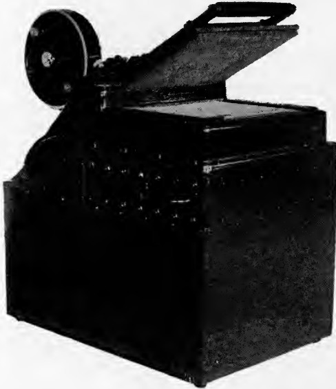
FIG. 1. Front view of camera, showing platen raised.
