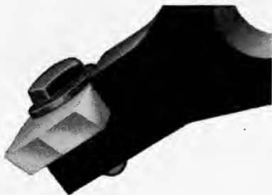
FIG. 7. Attachment of cutter to armature extension of sound recorder.
