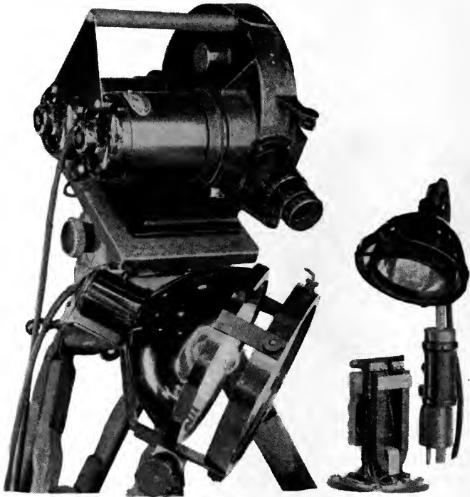
FIG. 4. Portable lighting units used for high-speed work.
