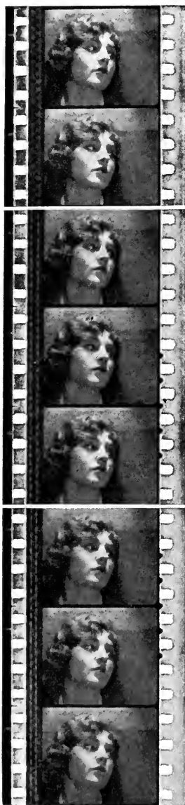
FIG. 5. Push-pull variable-density squeeze, showing full-width track, double squeeze of 6 db. and double squeeze of 12 db. ( Upper ) no squeeze; ( Middle ) 6 db. squeeze; ( Lower ) 12 db. squeeze.
