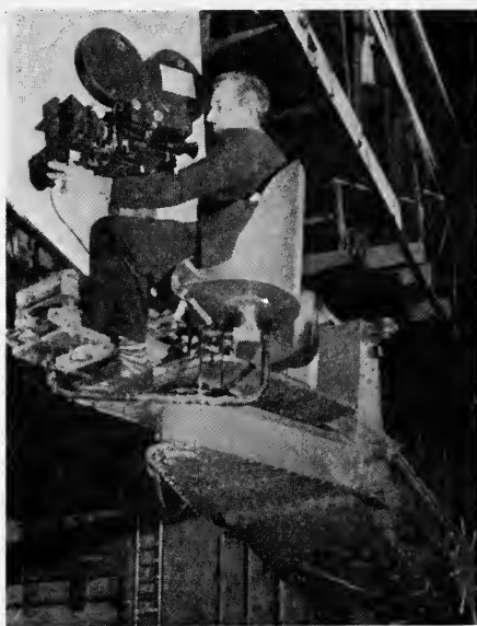
FIG. 10. Slater-equipped NC camera, on boom.
