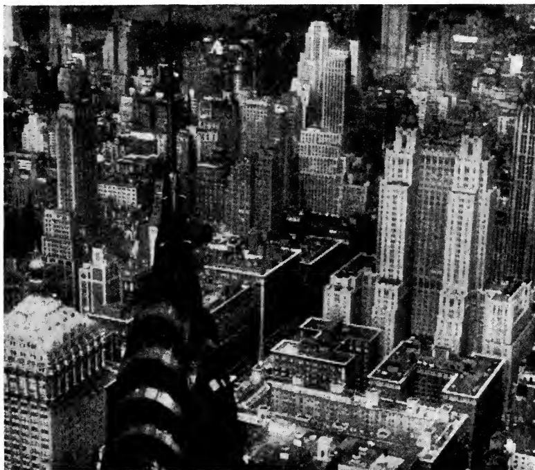
FIG. 16. Result of optically scanning original of Fig. 15 with a slit aperture to simulate a 441-line, 30-frame, 60-field image within a 4.25-mc band ( Goldmark and Dyer 7 ).
