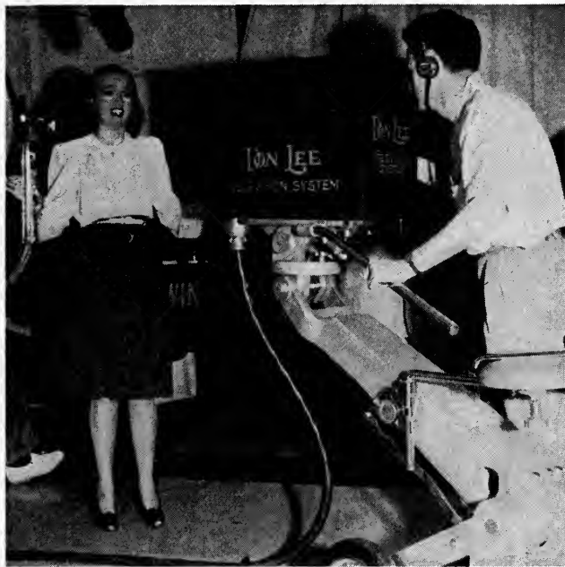
FIG. 1. The mirror-viewing camera-tube-image viewfinder. The cameraman is viewing the image on the photoelectric plate, with right hand on the focusing adjustment on the farther side of the camera. The left hand is used for panning and tilting as shown. The scene is a close-up. The exaggerated under-eye make-up is no longer used.
