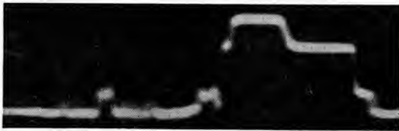
FIG. 5. Similar to Fig. 4, but showing line pulse and pedestal more clearly.
