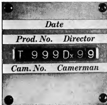
FIG. 6. View of slate-box face indicating information carried thereon.
