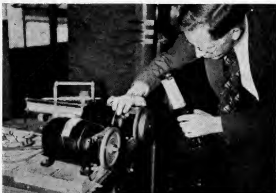
FIG. 9. Testing motors for stiffness and oscillation by means of stroboscope.
