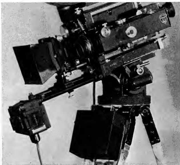
FIG. 9. Attachment shown mounted on open tripod set-up of NC camera.
