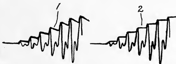
FIG. 18. Step effect on charging and exaggeration of same by discharge between input peaks.
