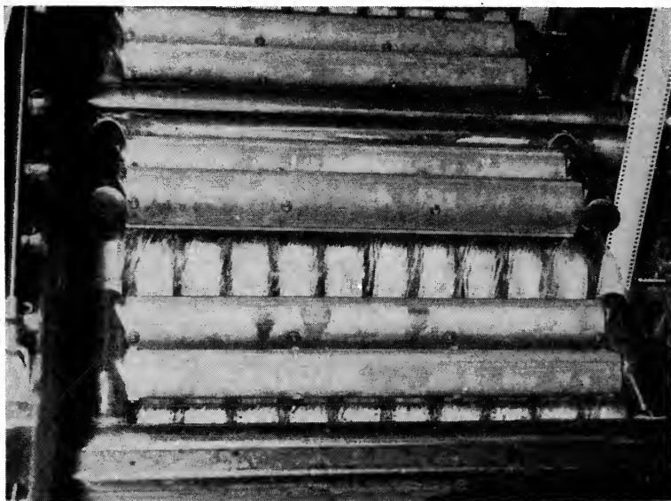
FIG. 6. Photograph showing the arrangement of the jets and the flow of developer on the surface of the film.
