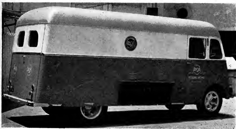
FIG. 4. Access to storage battery compartment is through 2 outside doors as well as from inside.
