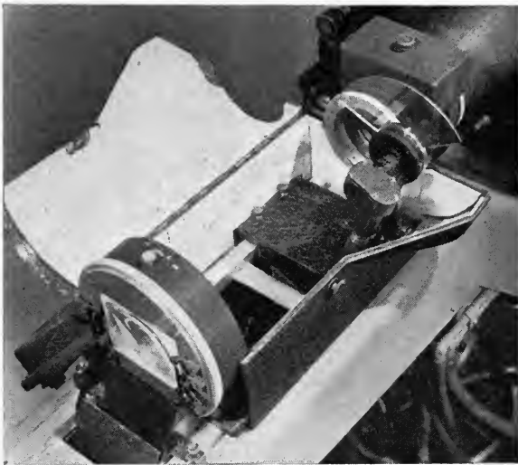
FIG. 3. Paramount transparency stereopticon, looking down on optical system showing water-cell, heat-resisting experimental glass shutter, and field condensing system for plates.
