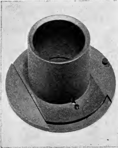
FIG. 2. Lamp base used for testing projection optical and illumination systems.
