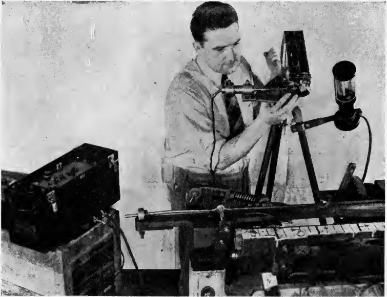
FIG. 11. Eastman Ciné-Kodak Special fitted with a stroboscope and set up to make a high-speed record of an action in the operation of a loom.
