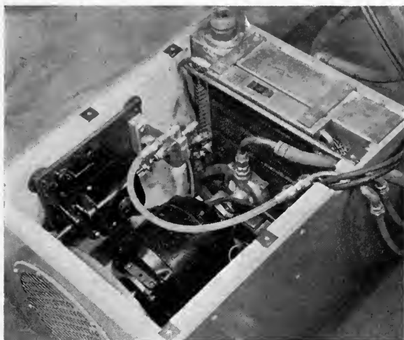
FIG. 2. Paramount transparency stereopticon cooling unit consisting of radiation units for water-cell and lamp water circulation.
