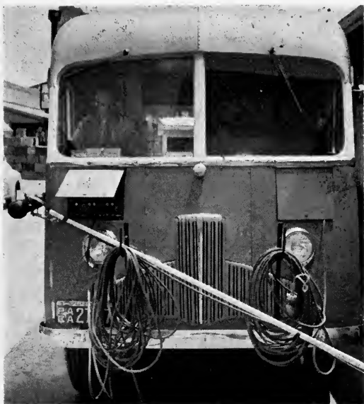
FIG. 10. Power outlet shown at right, compartment for microphone preamplifiers at left.
