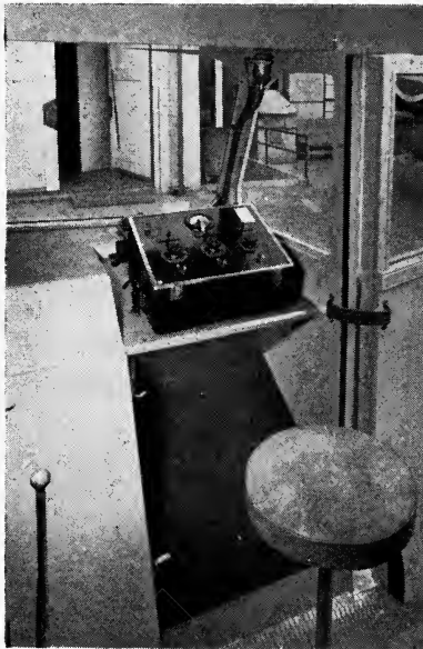
FIG. 9. Mixing panel in location setup position.
