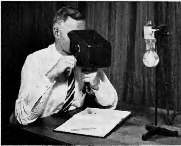
FIG. 1. Ashdown Rotoscope for making observations under conditions where light from subject being observed prevents the use of ordinary stroboscopic methods.
