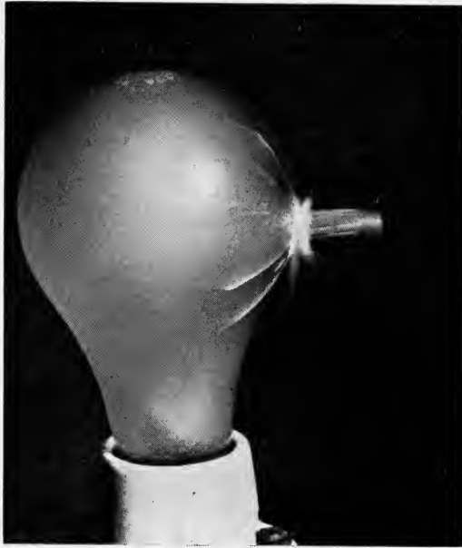
FIG. 5. Photograph of a 0.30-caliber bullet (velocity 2700 ft per sec) striking an electric lamp bulb. Note that the cracks in the glass travel faster than the bullet. An exposure of less than 2 \times 10^{-6} sec is required to "stop" the bullet without blur as shown in this picture.
