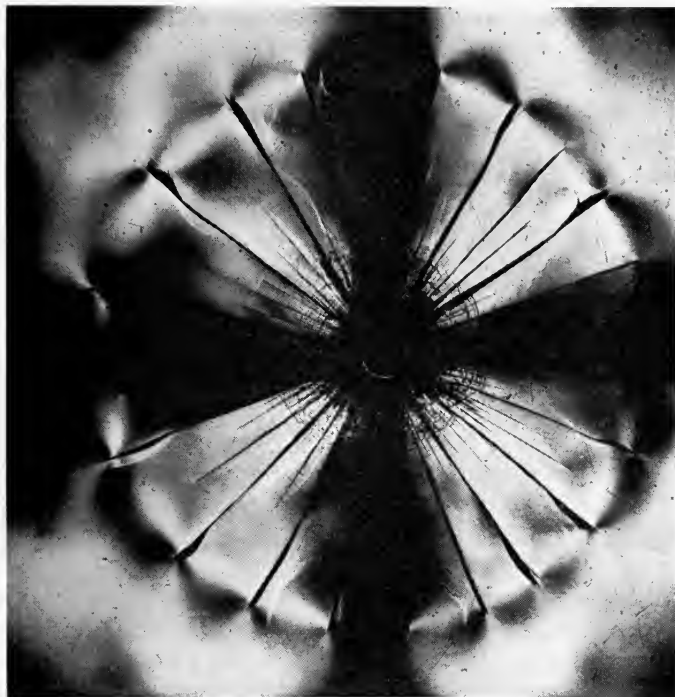
FIG. 6. A microsecond silhouette photograph taken with stroboscopic polarized light to show the stress pattern during the growth of the cracks in a glass plate when violently broken. The crack velocity is 5000 ft per sec. It is measured by taking 2 photographs spaced in time by 15 microseconds.
