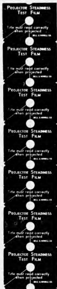
FIG. 1. Holes punched in film for testing projector steadiness.
