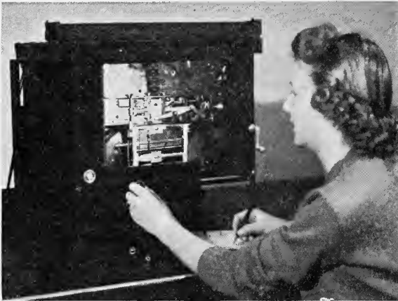
FIG. 4. The special projector for examination of motion picture film. Horizontal and vertical scales with movable transparent rulers permit measurements of positions of the subject to be made.
