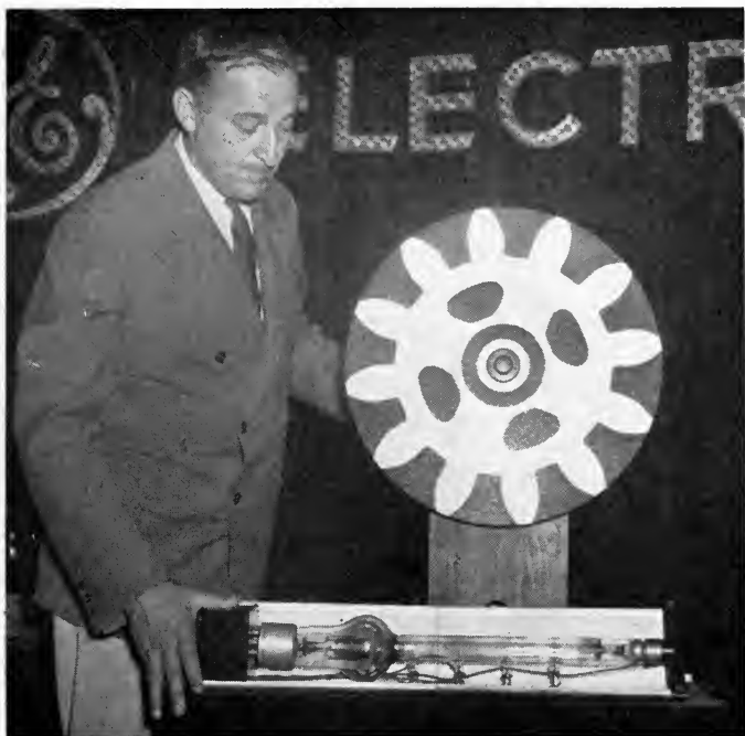
FIG. 2. Stroboscopic equipment used for demonstration purposes. In the normal operating position, the tube and reflector are turned toward the wheel. The useful light from the stroboscopic tubes originates either in mercury vapor or rare gases.
