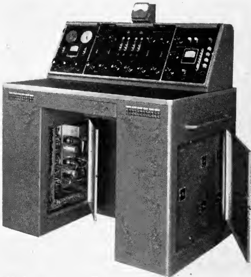
FIG. 11. Equipment may be serviced through panel doors on 5 sides of the console, two of which are shown.
