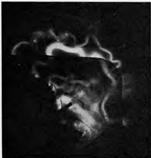
FIG. 8. High-speed multiple-exposure photograph of arc interruption, showing successive stages of the arc at intervals of about 1/300 of a sec.
