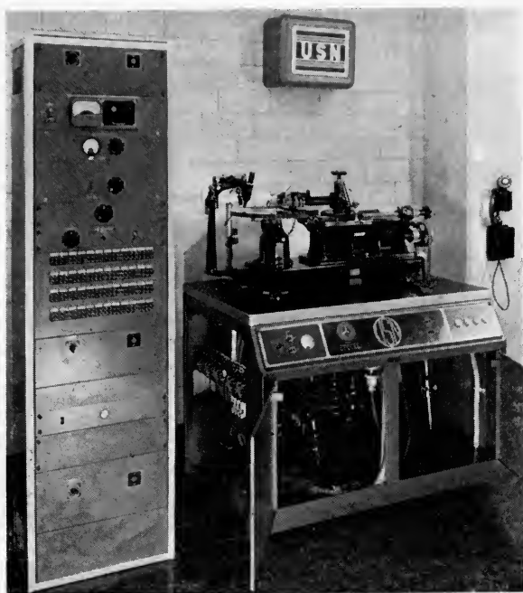
FIG. 16. Disk recorder, table, and associated equipment, showing accessibility for servicing.
