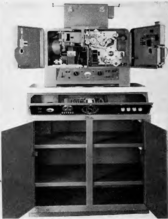
FIG. 15. All switches, meters, and other equipment are readily accessible on hinged panel.
