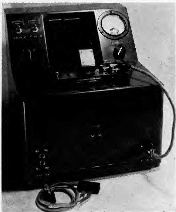
FIG. 24. Light-valve projector, showing ribbon image on rear screen.
