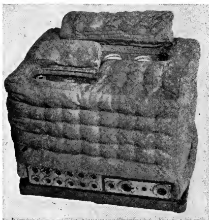
FIG. 6. Recorder equipped with insulating cover for low temperature operation.
