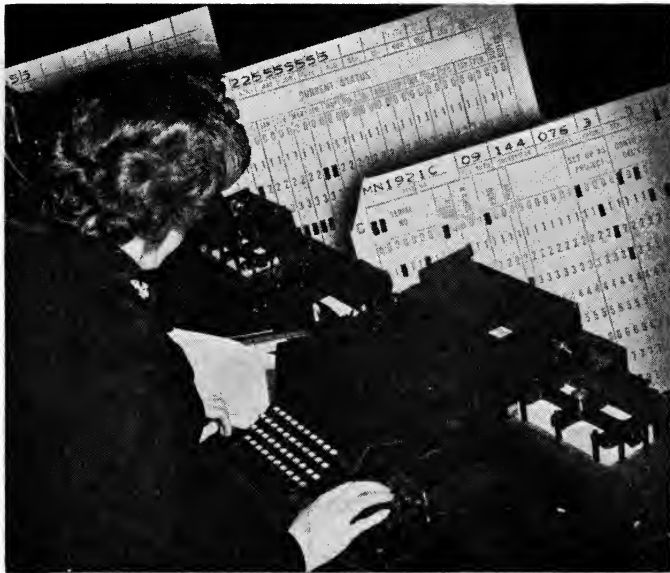
FIG. 2. Converting data furnished by Training Film Branch into punch-card form.
