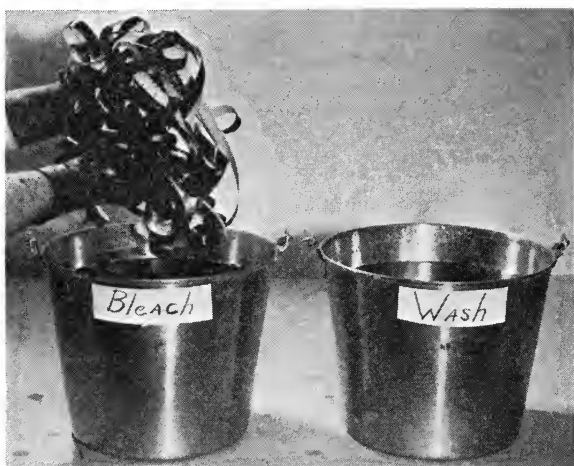
FIG. 8. Sixteen-millimeter "bucket" process—transferring mass of film from one solution to another, using rubber gloves.
