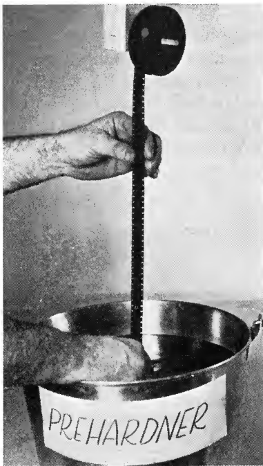
FIG. 7. Sixteen-millimeter "bucket" process—winding dry film into prehardener solution.
