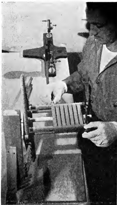
FIG. 5. Loading 16-mm rack for 8 × 10-in. cut film tanks.
