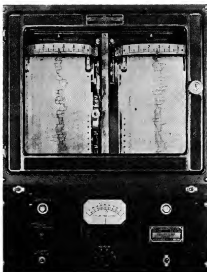
FIG. 3. Philips direct-reading frequency meter installed on rack and driving a 5-ma recorder without an auxiliary amplifier.
