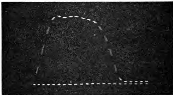
Fig. 7—Curve produced by the shutter of a 24-inch focal-length K-18 aerial camera at the maximum aperture of f/6 .
