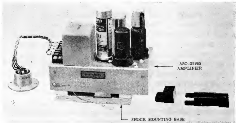
Fig. 14—RA-1278 phototube monitor unit—assembly.
