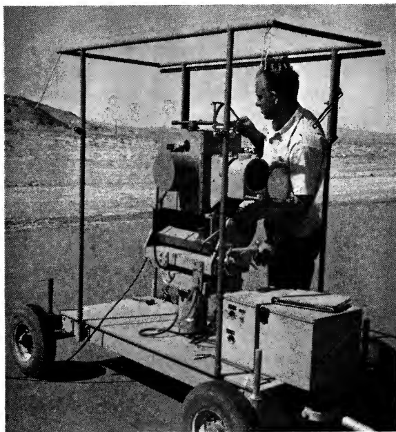
Fig. 4—Operator of a Bowen ribbon-frame camera orienting the camera in respect to the trajectory by use of a gunner's quadrant. The small telescope on top of the camera is used for setting one of the needed angles.
