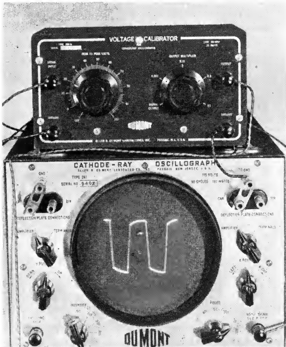
Fig. 11—Typical photograph of apparatus with oscillogram using double-exposure technique.
