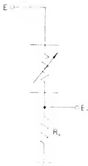
Fig. 2—Simple signal circuit using photoconductive cell as detector; signal voltage is developed across the resistor R_0 .
