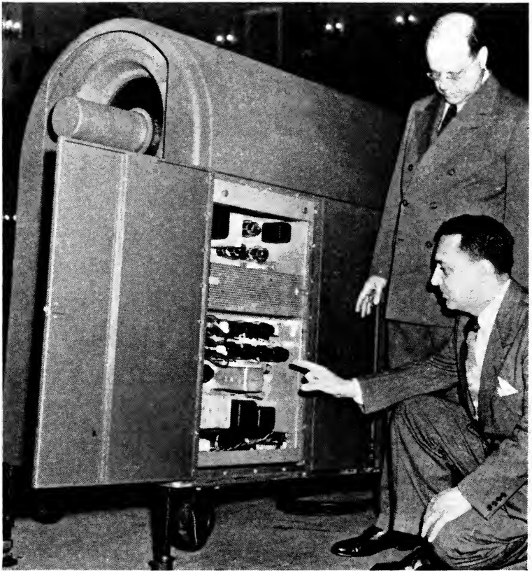
Fig. 2—Projector with 20-inch mirror and 21-inch plastic lens, demonstrated in 1948 at TESMA Convention, St. Louis.
