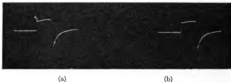
Fig. 28—Same oscillogram with bright and dark markers. (Note how overshoot is missing because of dark markers in (b).)
