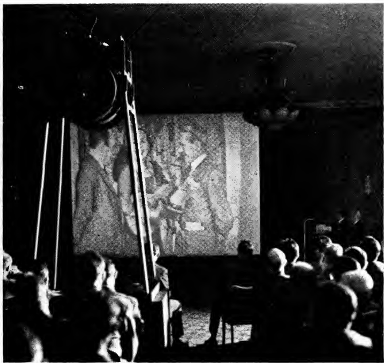
Fig. 7—Equipment used in the demonstration at the Hotel Statler ballroom with an actual television picture on the screen. The picture originated in an anteroom of the ballroom and was fed to the television projector by direct cable connection.
