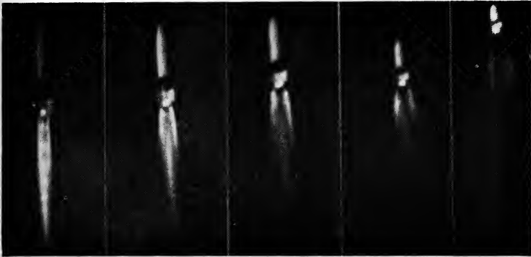
Fig. 8—Sample frames at 10-second intervals of tracking telescope record of A-4 missile during period of propulsion, showing changing jet structure. Corresponding slant ranges vary from 8 to 20 miles.
