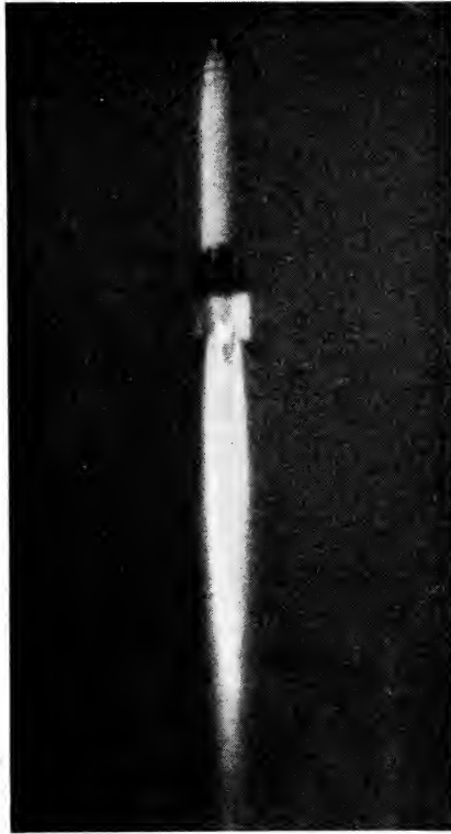
Fig. 7—4.5-inch tracking telescope photograph of A-4 missile, at a distance of 8 miles, taken with a 20-foot focal length. Not reproduced portion of 35-mm frame contains azimuth, elevation, and time records.
