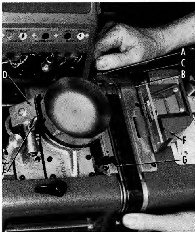
Fig. 6. Close-up of picture film trap, showing method of threading film.
