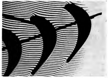
Fig. 24. Flow past cascade of turbine blades.
