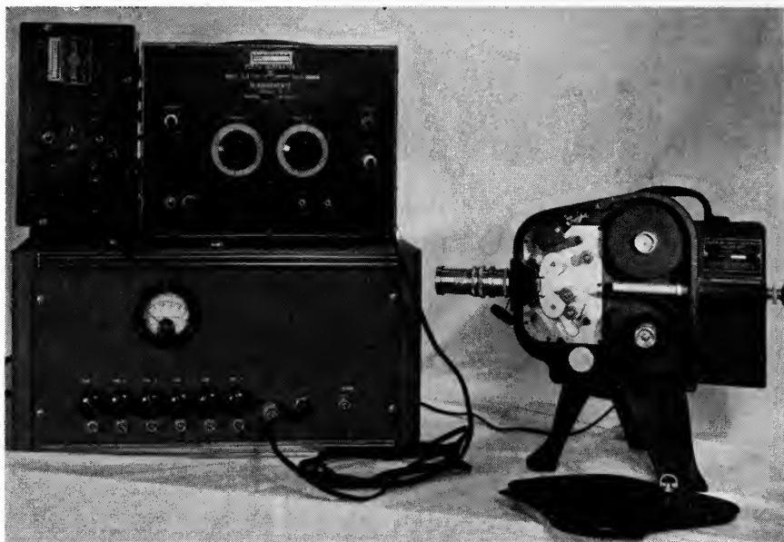
Fig. 1. Pulse timing system and neon timing light mounted on upper sprocket clamp of an Eastman High-Speed Camera.
