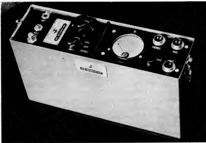
Fig. 3. Mite recording amplifier showing control panel and input and output receptacles.
