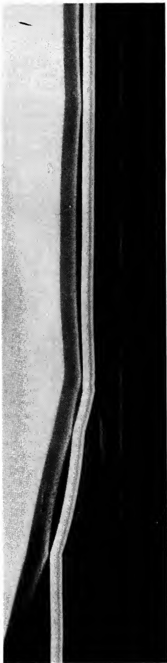
Fig. 3. Streak image of punch displacement.
