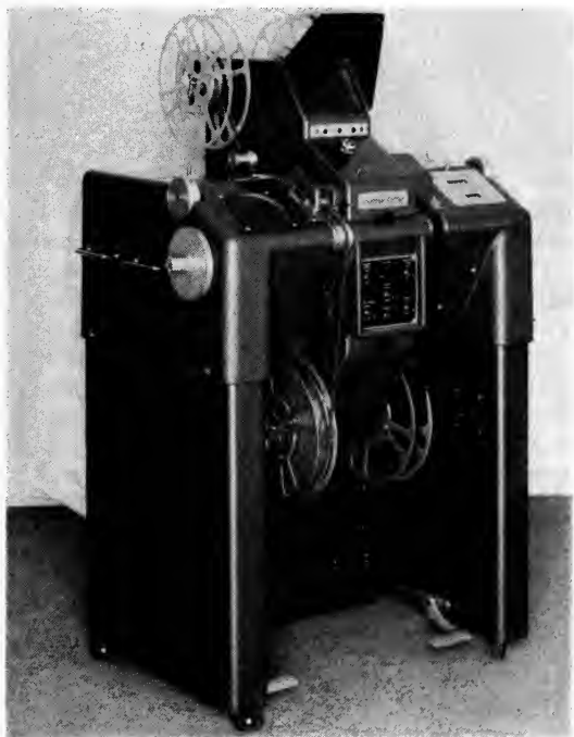
Fig. 1. Front view showing operation with film reels and bag at the rear for collecting film if reels are not used.
