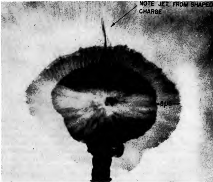
Fig. 17. Shock wave and the explosive products which come from a dynamite cap.
