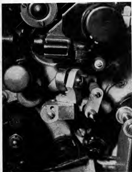
Fig. 1. Record-playback head installed in projector. Note angular position of head.
