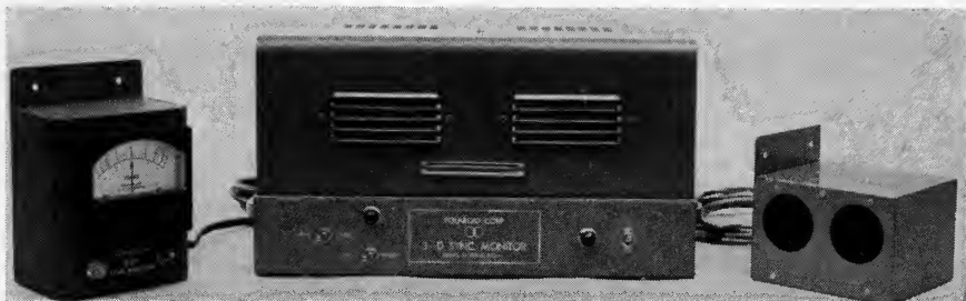
Fig. 1. Showing the Polaroid 3-D Electronic Sync Monitor, Model 21. The meter is at the left, and the photocell housing is on the right. The main electronic chassis (with 18 tubes and 5 relays) is in the center.
