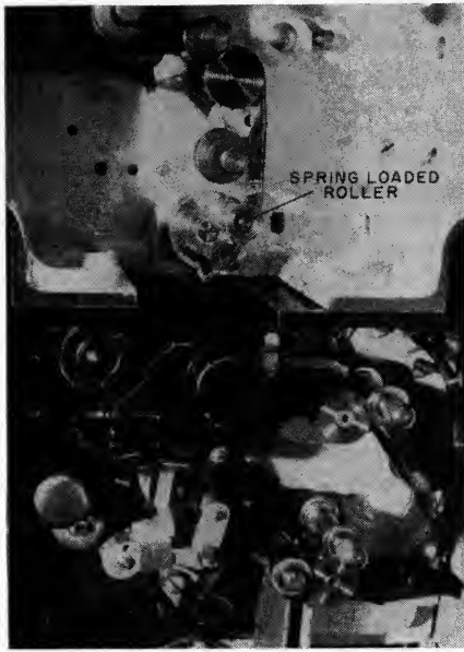
Fig. 9. Spring-loaded roller installed to add tension to film.
