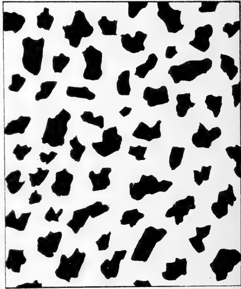
Fig. 3. Diagrammatic representation of a ferrospor: iron scattered, or sporadic, in a continuum of silicate.
