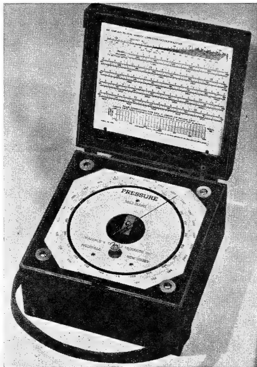
Fig. 4.—Aneroid barometer, range 610 to 1,085 millibars. Pointer makes two revolutions; scale 7\frac{1}{2} inches in diameter. The humidity and correction factor is obtained from the nomogram at the top of the cover; the conversion of pressure to altitude in the SMT standard atmosphere is given in the chart in the middle; and data on the temperature error of the barometer can be plotted on the graph at the bottom.
