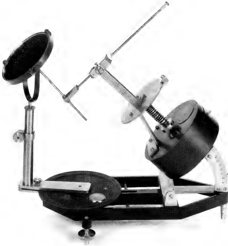
Figure 21. A "Keith American Heliostat" made by Edward Kübel for Samuel P. Langley's experiments with solar radiation. Signed on hour dial and twice on base "Edward Kübel Math. Inst. Maker Washington, D.C." National Museum of American History, Cat. No. USNMo 211,531.
