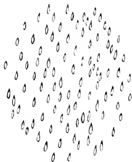
Fig. 1. Etch-figures on babingtonite, produced by action of hydrofluoric acid. Magnification 250\times .
