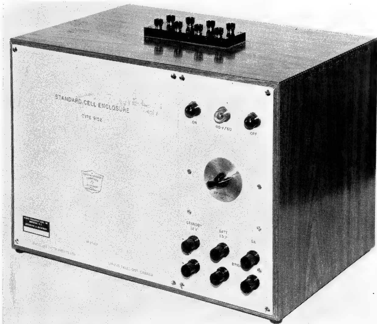
Fig. 4. A constant-temperature controlled box for saturated standard cells.
