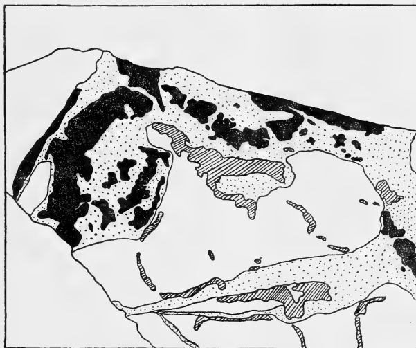
Fig. 1.—Iron sulphide (marcasite after pyrite) veins (black) with some barite (lined) associated with siderite-rich mudstone (dotted) and clay mudstone (white). Camera lucida \times 4 .
