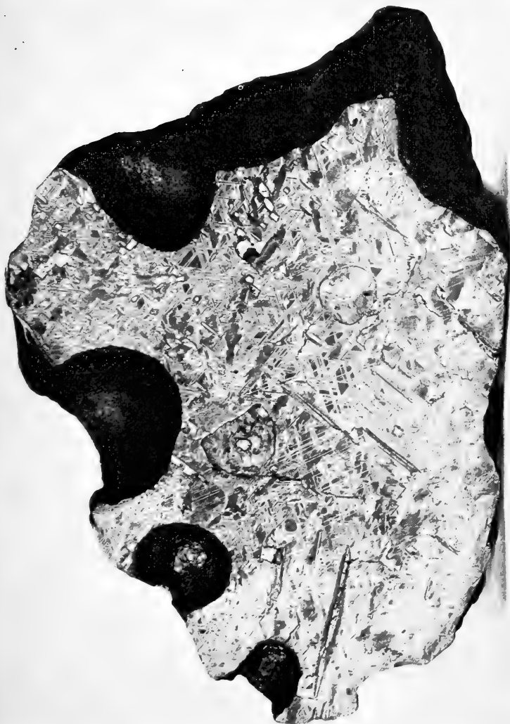
a Section 8. \frac{1}{4} nat. size. Etched by bromine water.
