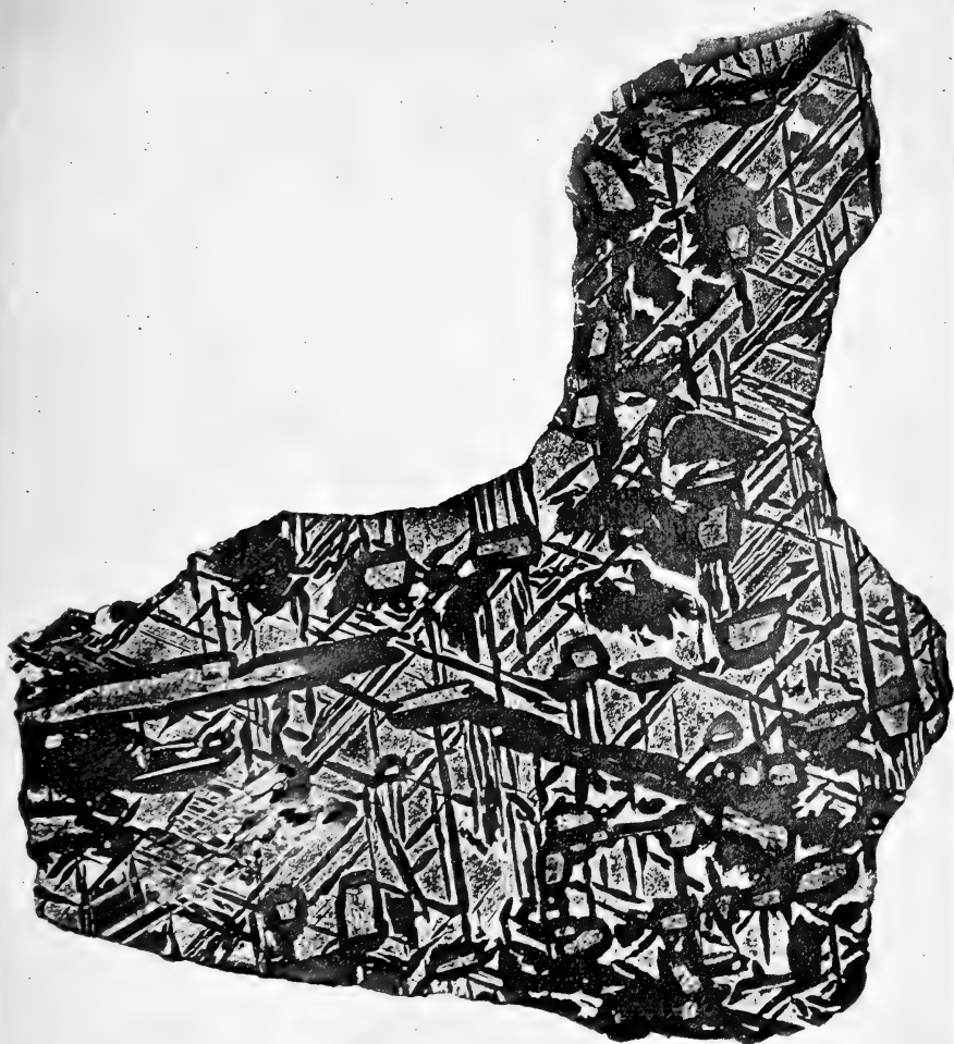
Section 1. Enlarged 2 dias. Etched by bromine water.
