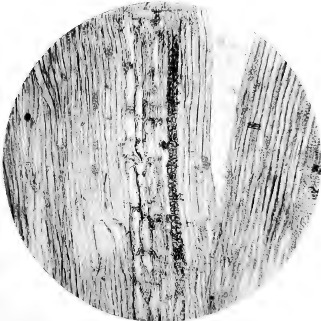
Flindersia australis .—Radial section showing a conjugate crystal parenchyma with a calcium oxalate crystal in each cell; to the left, wood parenchyma, the remainder fibres. ×100.
