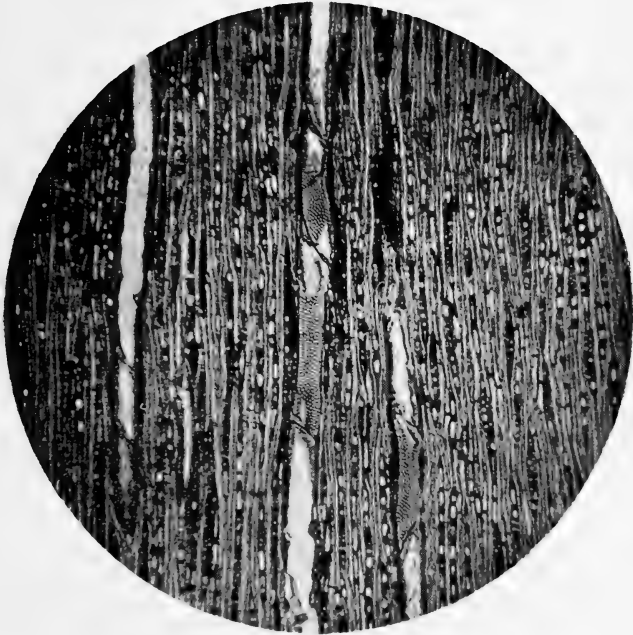
Mallotus philippinensis. —Showing end view of rays with crystals. \times 45 .
