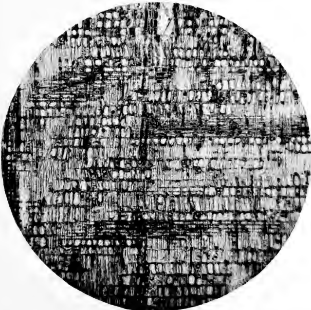
Mallotus philippinensis. —Radial section showing heterogeneous ray parenchyma with two or more crystals in an individual cell. \times 45 .
