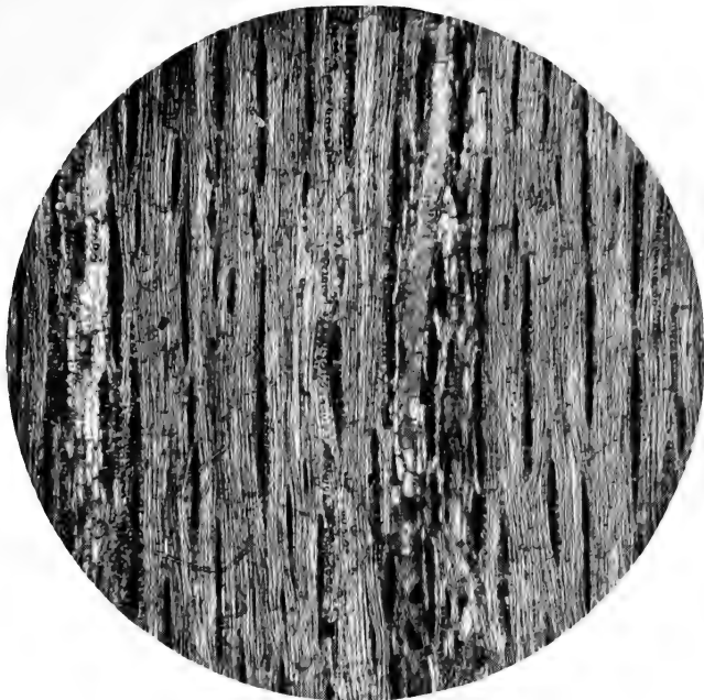
Acacia pendula. —Tangential section showing numerous wood parenchyma with crystals. \times 45 .
