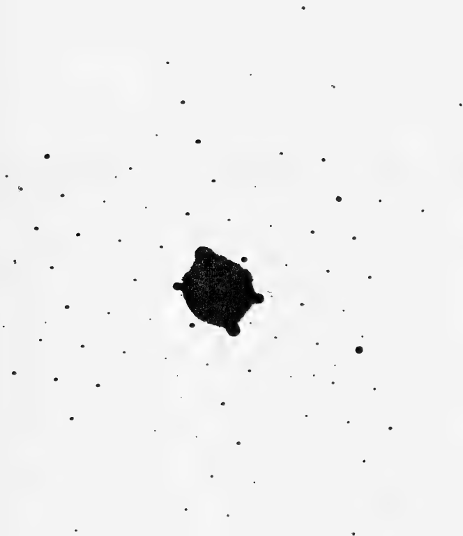
Fig. 5.—Cross-grating pattern from crystal of boric acid.
