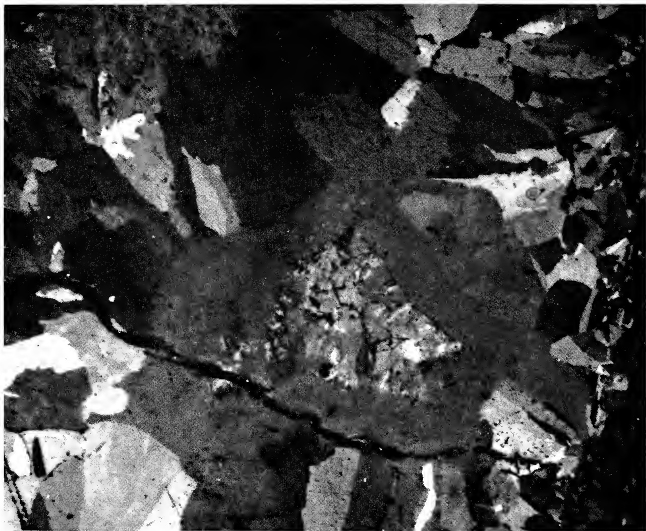
PLATE II.—Massive marcasite with minor pyrite. Cell structure is present on the right-hand margin of the field of view. Reflected light, oil immersion, crossed nicols. \times 230 .
