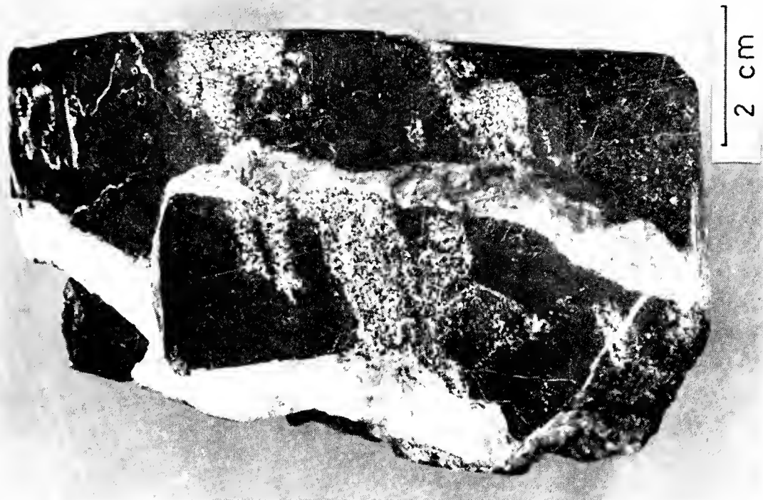
FIG. 2.—Rodignite veins (white) transecting and offsetting schlieren-banded (spotted and streaky) chromitite (chromite with serpentine minerals) and massive chrome ore (black) from the Mooney Trig Mine, North Mooney Ridge.
