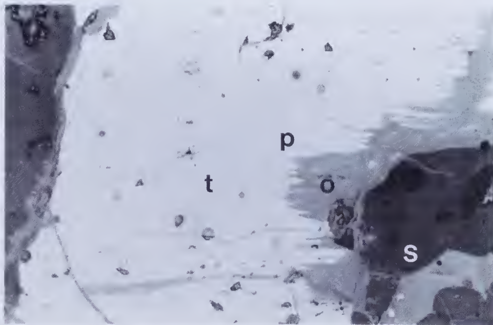
Figure 4. Extensively weathered particle of troilite (t) with dark grey iron oxides (o) surrounded by silicates (s). Weathering of troilite has progressed along (0001) parting planes and there is incipient development of pentlandite (p). Field of view 0.2 mm.
