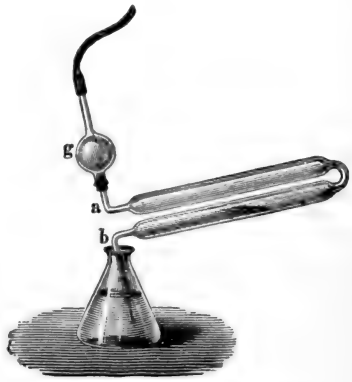
FIG. 39.—Method of filling a density tube having a fine bore.
