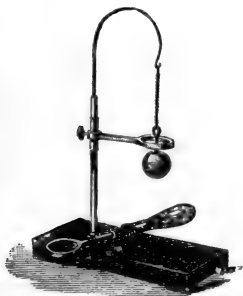
FIG. 55.—Apparatus for showing that a metal ball is larger when hot than it is when cold.
