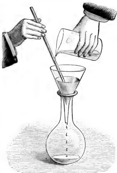
FIG. 72.—How to pour a liquid into a paper filter in a glass funnel.
