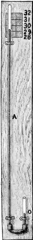
FIG. 50.—The pressure of the air on the mercury in the small tube is able to keep up the column of mercury in the long tube.
