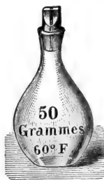
FIG. 37.—A bottle for determining relative density.
