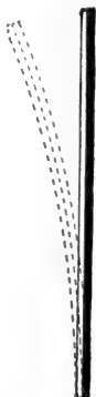
FIG. 56.—Compound strip of ebonite and wood to show the greater expansion of ebonite when heated.
