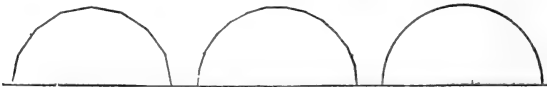
FIG. 2.—To illustrate how a curve may be considered to be made up of an infinite number of short lines.
