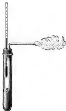
FIG. 63.—Test-tube with thermometer fitted for observing the boiling point of water.
