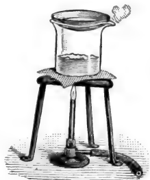
FIG. 78.—The shallow basin has solution in it and is kept hot by the steam rising from the water in the glass beaker.
