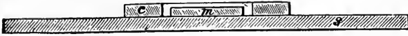
FIG. 130.—Section through a Thoma-Zeiss Hemacytometer. S , Glass slide; m , ruled stage; c , support for cover glass, 0.1 mm. above the stage.
