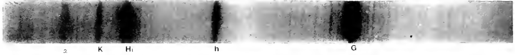
SPECTRUM OF ALTAIR, taken by the BROTHERS HENRY with a Flint Glass Prism of 45°
