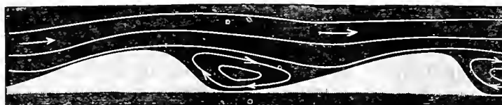
FIG. 1.—Action of Current upon Ripple Mark.
