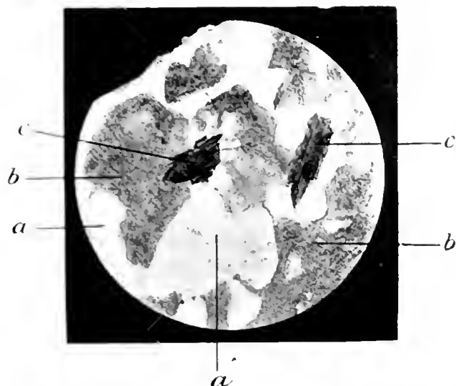
A Section of Granite from Skiddaw, \times 15 . (Reproduced from a slide in the Woodwardian Museum, Cambridge, by kind permission of Prof. T. McKenny Hughes, F.R.S.) A, Quartz; B, Felspar; C, Mica.
