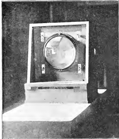
Fig. 1.—The 12-inch Taylor Photo-visual Lens and Support for forming the Solar Image on the Primary Slit of the Spectroheliograph.
