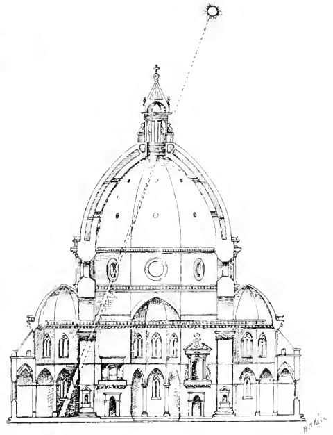
Fig. 4.—Section of the dome, showing the path of the sun's rays at the summer solstice. (After Nimenses.)
