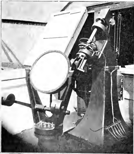
Fig. 2.—General View of the Large Siderostat showing the 18-inch Plane Mirror. The upper portion of the House is here moved on its rails towards the north.
