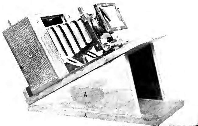
Fig. 2. The grating attached to a 5 by 4 Kodak Camera.
