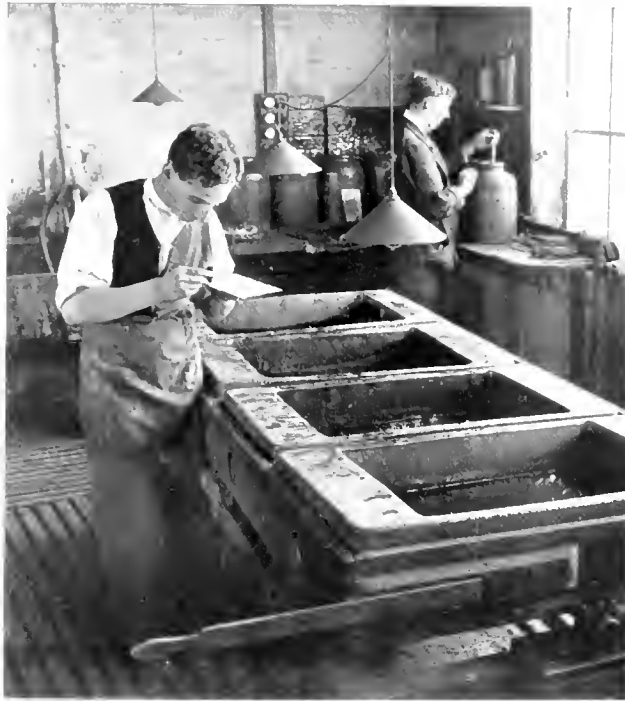
FIGURE 8. The Etching Bath. Examining the plate for depth.
