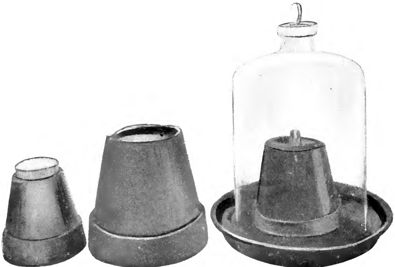
FIG. 31.—MOIST-CHAMBERS FOR GEOTROPIC EXPERIMENTS. One-fourth the true size.
