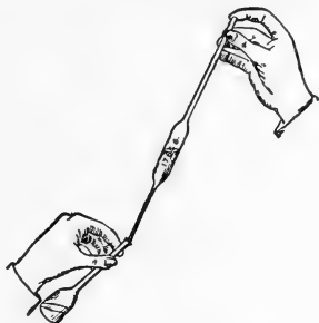
SHOWING PROPER WAY TO ADD THE MILK TO A TEST BOTTLE.— Courtesy De Laval Separator Co.
