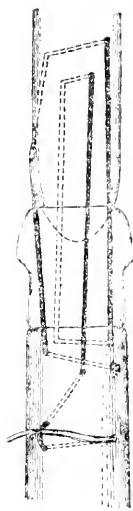
Figure 16. Manner of attaching the two principal parts of the harpoon. From Boas, The Central Eskimo , Fig. 420, p. 489.
