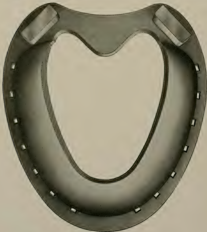
Fig. 35—Inferior (convex) surface of Cochran shoe.
