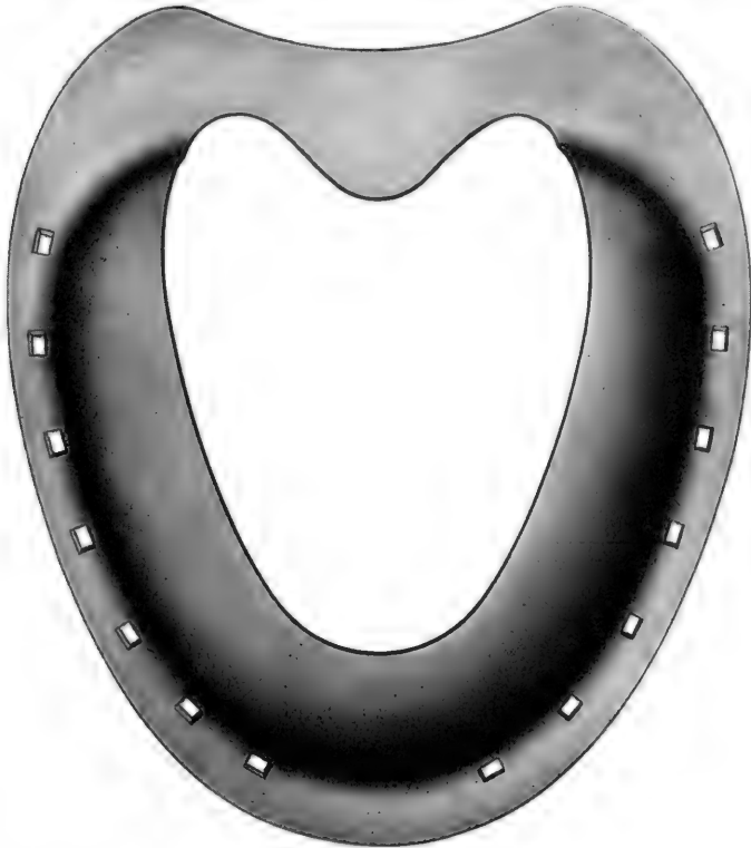
Fig. 36—Superior surface, showing concavity or bowl, as formed by the toe and branches of the shoe, as designed by Dr. David W. Cochran.
