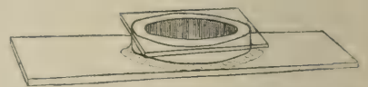
Slide, cell, and covering-glass square in readiness for placing in the incubator.
