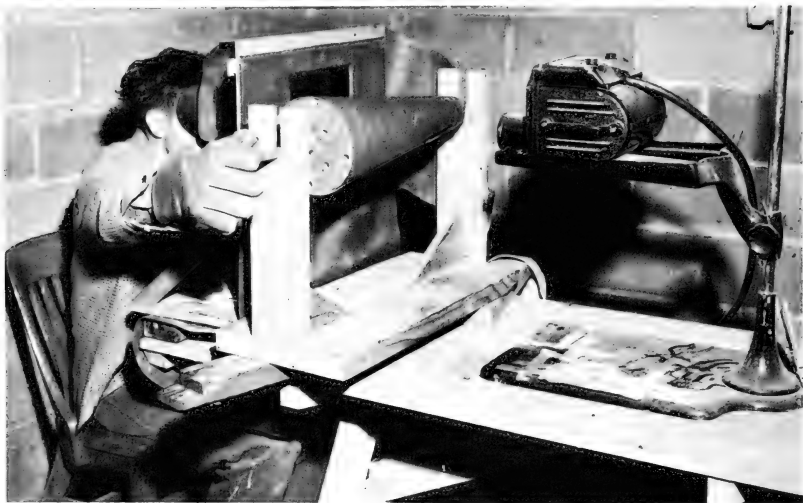
Fig. 9. -- A fluoroscope unit used as an aid in determining the incidence of ingested commercial shot pellets in live-trapped waterfowl. Ducks were placed in the cone shown in the illustration and rotated before the fluoroscopic screen. By this method a technician could recognize and locate the position of lead shot within the body of a duck.
