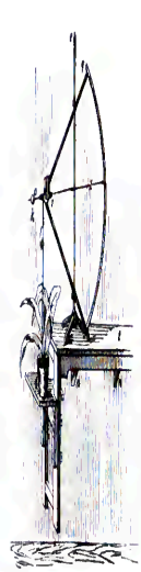
Fig. 83. Simple auxanometer. After OREWICH (Smaller Practical Botany, 1909).
