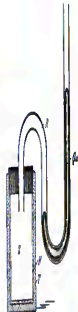
Fig. 3. Pfeffer's osmotic cell. A, porous pot; B, precipitation membrane; C, manometer containing mercury; D, Z, sugar solution.
