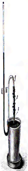
Fig. 12. The glass tube, g , is fixed by means of rubber tubing, c , to the stump of a Cecidix , a , and filled with water ( W ) and mercury ( H ). (From the Rein Textbook .)
