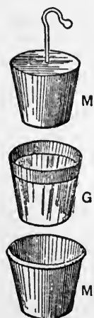
FIG. 6.—Leyden jar with removable coatings. M M, metallic cases; G, glass jar.
