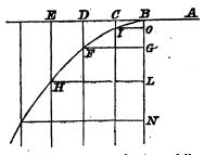
tal motion. "A B represent a horizontal line or plane placed on high, on which let a body be carried with an equable motion from A towards B, and the support of the plane being taken away at B, let the natural motion downwards due to the body's weight come upon it in
