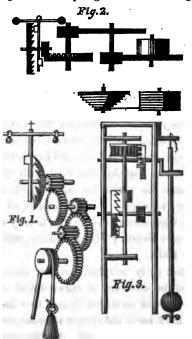
beginning of its motion." This contrivance of the chain is mentioned by Cardan, in 1570, and is probably still older. In both figures the name given to the cross bar, with the weight attached to it, is "the time or balance, (tempus seu libratio) by which the motion is equalized."
