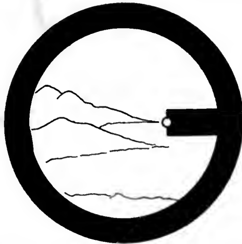
Fig. B. From Galton's original drawings for his heliostat. Field of view of the telescope with the mock-sun covering the point of a promontory to which the instrument would flash light.
